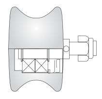
Used extensively on overland conveyors with horizontal curves, to prevent the belt transversely riding up over the trough and/ or return idler sets.
