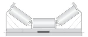
Used to train the belt approaching the head end of the conveyor.
